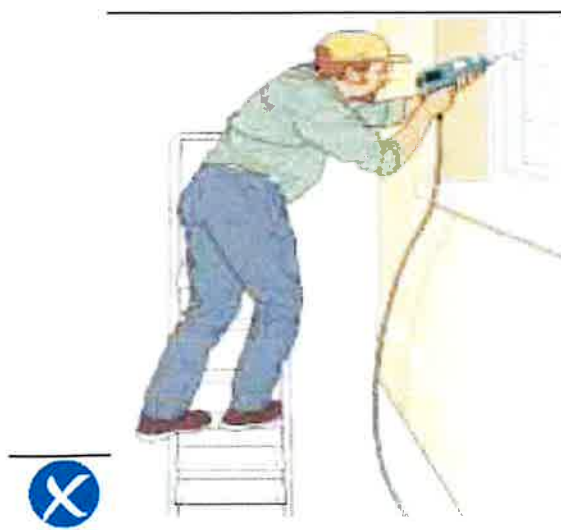
Incorrect – steps side on to work activity
